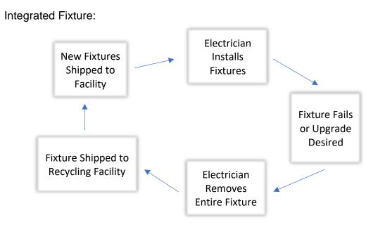
Assuming a comparable quality of product (5-year warranty integrated fixture and 10year warranty tubes), the initial cost is greater for integrated fixtures. A two-foot by fourfoot troffer (\$52) with three top-of-the-line (with a 10-year warranty) 11W 1,540-lumen tubes (\$11 each) comes out to \$85, while an integrated fixture with similar design and performance ratings is \$90.
