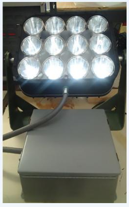
Under contracts with Stennis Space Center, Energy Focus designed LED floodlights that could withstand conditions inside a rocket engine test stand and would not pose a hazard themselves.
